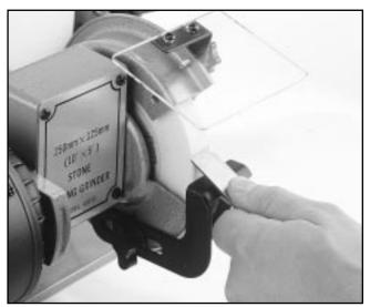
Figure 4. Proper grinding positioning.
